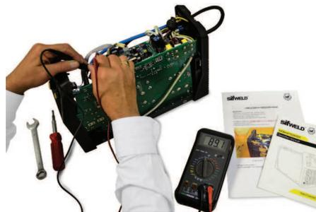
equipment or a welding system (including wire-feeder) conforms to the required operating specification. Incorporating Accuracy Tests (the closeness of measurement to the defined or true value) and/or Consistency Tests (the repeatability of the equipment output over time). These operations result in a Validation Certificate.
