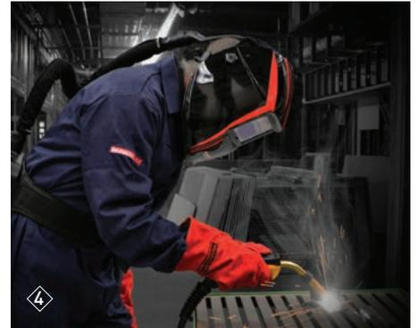
that provides a 2-speed clean air and an 8-hour battery life from a full charge. Fully CE rated to EN 12941 TH2, it includes a multi functional helmet providing full-face protection, with shade 9-13 auto-darkening lens. The lens has a fast reaction time of just 0.3ms!
