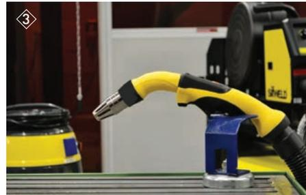
balances pressures to prevent disruption of the shielding gases. You can therefore use the same shielding gas flow rates as with a standard MIG torch.
