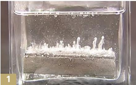
**FIGURE 1. HYDROGEN ESCAPING FROM A WELDMENT.**
