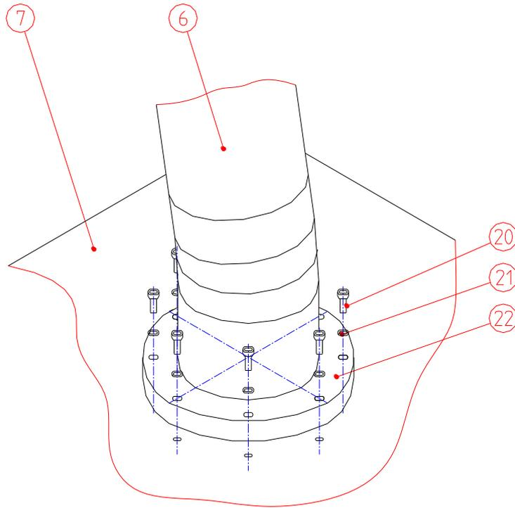
The extractor fitting (e.g. an extractor hose or an extractor arm) must be mounted on the extractor spouts or the housing cover.
