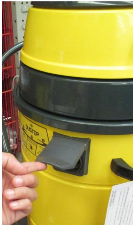
Once the cleaning process has finished, remove the cap from the suction inlet and connect the accessories to continue the vacuum process.
