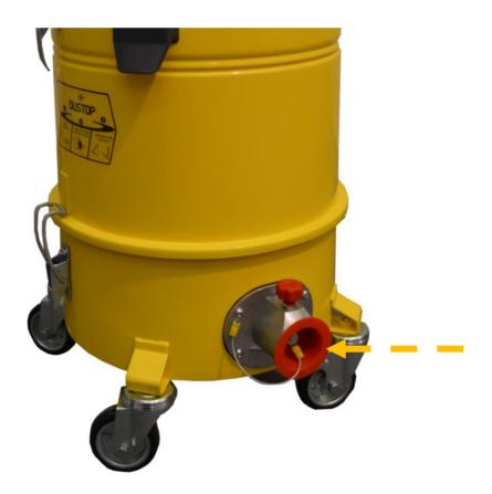
Open the flap as indicated in the picture below allowing the air to flow into the filtering chamber thus providing a counter air flow that passes through the filter. Repeat this operation for at least 5 times.
